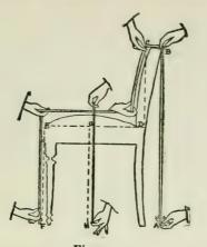
Figure 1. This sketch shows the method of measuring a chair to figure the yardage required for a slip cover.
